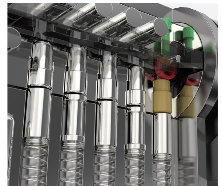
Inserted with the right key with roller. The roller will be pushed by the green pin and work with the yellow key pin.
